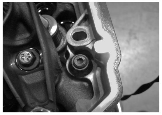
Finished machine work should allow easy removal and installation of the head stud.  $_{\rm REV\,1\,NOV\,2017}$
