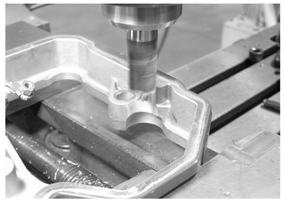
Remove material as necessary to allow clearance for the stud, nut and washer.
